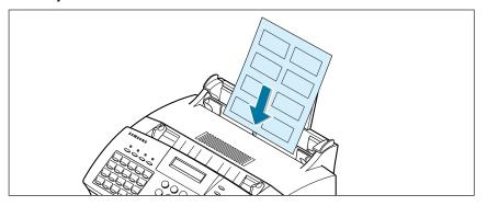
• Load a sheet of the card stock with print side up, short edge first.
